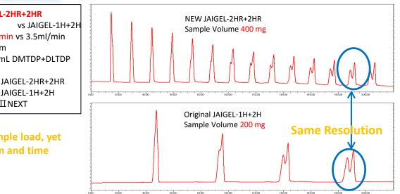
Colunm : JAIGEL-2HR+2HR Flow rate : 14ml/min vs 3.5ml/min Eluent: Chloroform Sample: 100 mg/mL DMTDP+DLTDP Injection Volume 400 mg / 4 mL to JAIGEL-2HR+2HR 200 mg / 2 mL to JAIGEL-1H+2H Detector : RI-700ⅡNEXT
